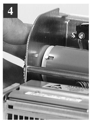
Manually turn the Spur Gear until the slots on the core engage with the lugs.
